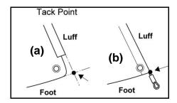
**G.4.1.8** Only the following **clew** construction arrangements are permitted for jibs **certified** after January 1st 2017.
